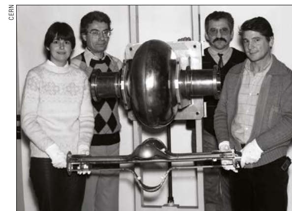
Fig. 2. The first prototype niobium-copper superconducting cavity, pictured in December 1983 with Nadia Circelli, Cristoforo Benvenuti, Jacques Genest and Max Hauer.
