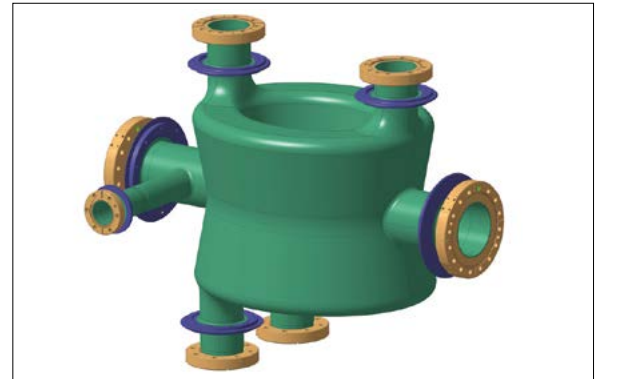
Fig. 2. Schematic view of the interfaces of two cavities under development: RFD (top) and DQW (bottom).
