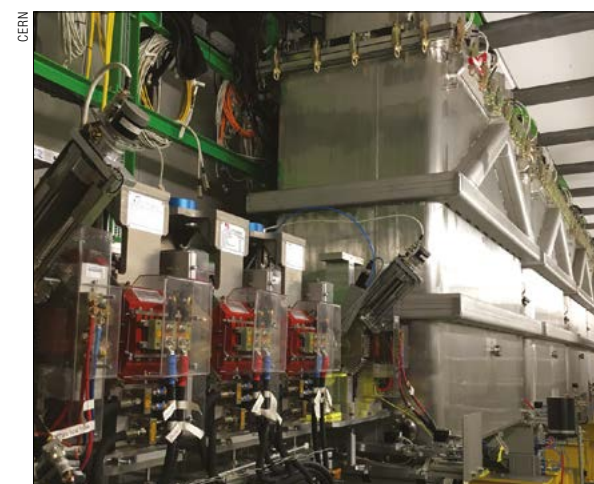
Fig. 3. The HIE-ISOLDE linac, which was completed this year and comprises 20 niobium-copper sputtered cavities hosted in four cryomodules operating at 101.28 MHz and 4.5 K.
